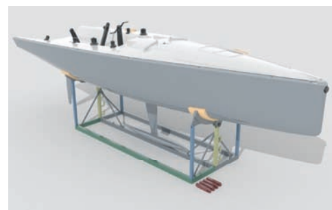
Sitting in her bespoke cradle, the Farr 400 has keel and rudder removed for storage
