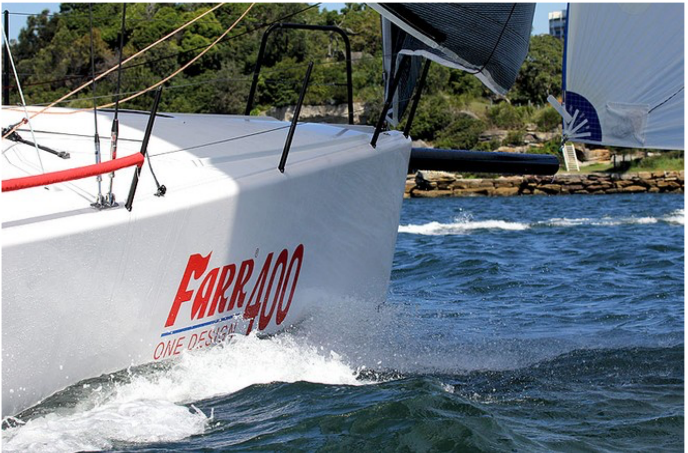
Full volume for'ard ensures bow gets up and you fly forward. - Farr 400 © John Curnow
